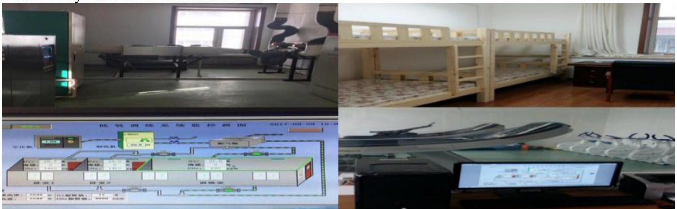
Fig.1. Simulated plateau training atmospheric hypobaric chamber
