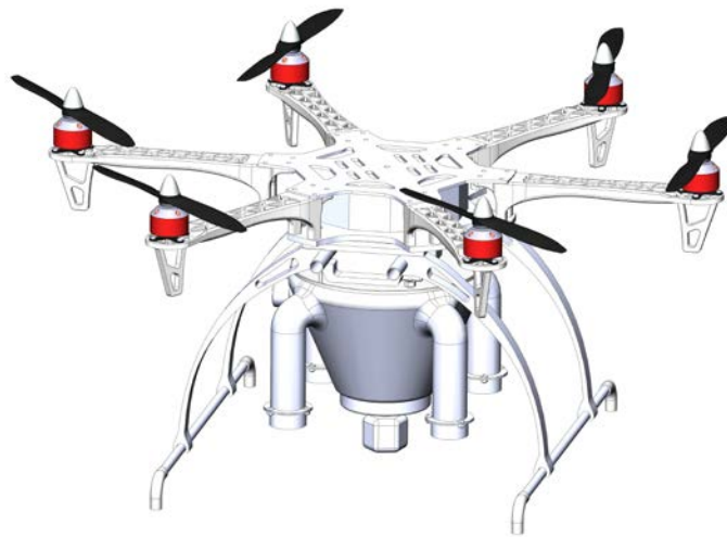
Figure 6. The Application of the Powder Spraying Device on the Plant Protection UAVs
